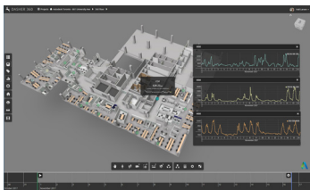
Figure 6: Air quality data visualized in the context of the 3D model of the Autodesk office in Toronto.
